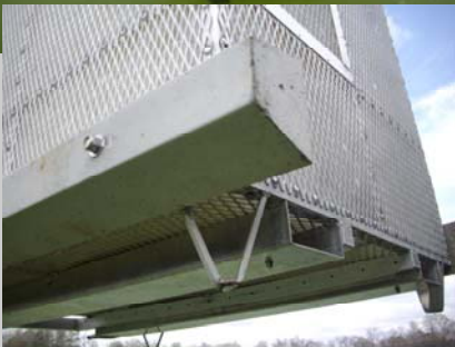
Dual Diffusion System for Easy Backflush of Media Bed
