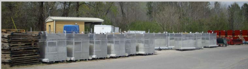
Dual Diffusion System for Easy Backflush of Media Bed
